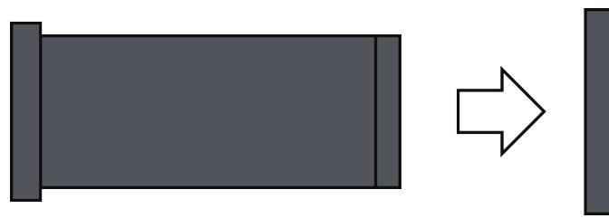
Step 2: After removing the handlebar grip, insert the MT611 into the handlebar.
