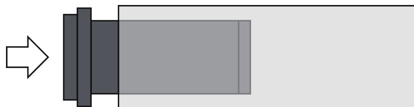
Step 3: Reinstall the handlebar grip.
