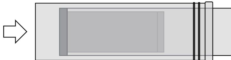
**NOTICE:** When the internal diameter of the handlebar is greater than 20mm, a spacer must be added to prevent the MT611 from sliding too far into the handlebar, which could affect antenna performance. After adjusting the device to the appropriate position, reinstall the cover.
